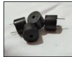
Gambar 2. 3 Buzzer Arduino
